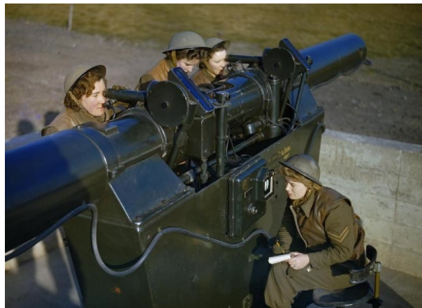
ATS crews "man" the optical rangefinder (above) and the mechanical range computer (below). The firing solution was fed to the gunners on dials and manually matched.
