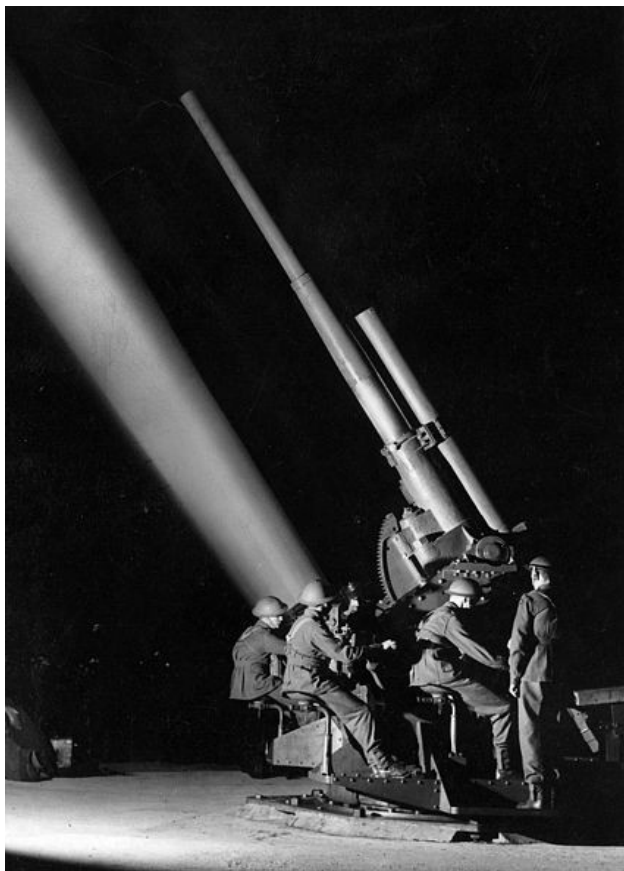
An anti-aircraft gun crew training with a searchlight and a QF 3.7-inch anti-aircraft gun. This gun was the mainstay of British heavy AA for the duration of WW2
